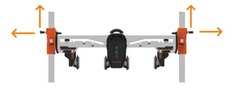
3. Remove 2 x Frame Locking Plates by unscrewing the 8 x wing bolts, by hand from either side of the ForceFrame. Place Frame Locking Plates and wing bolts to the side
